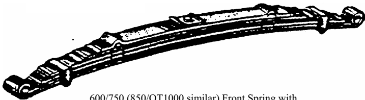
600/750 (850/OT1000 similar) Front Spring with main leaf flipped over & reverse-arched to lower suspension (compare to std. Spring with eyes facing down in fig 20a)
